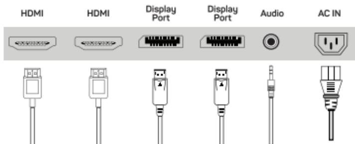
Connect the power cord for your monitor to the AC IN port on the back of the monitor.
